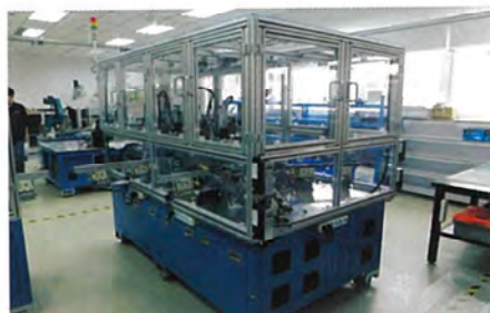
高精度检测设备 High-Precision Inspection Machine for PCB Side Connectors
